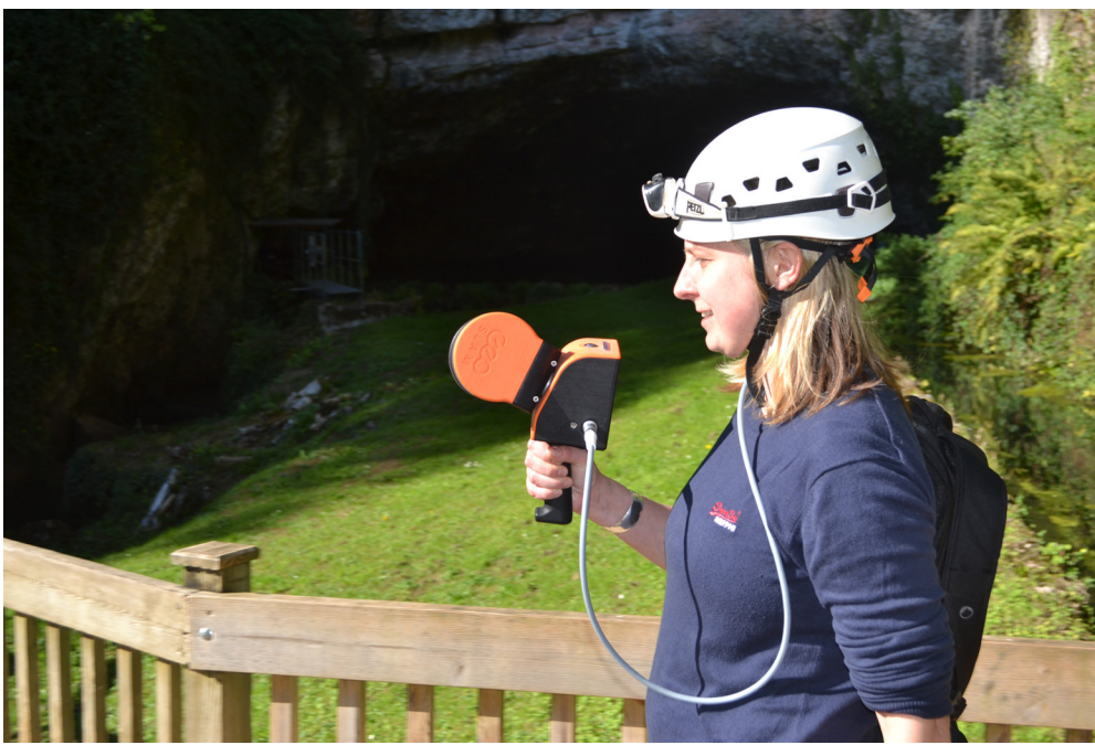
With no reliance on GPS, the ZEB-HORIZON is ideal for scanning in remote areas, or even underground environments
